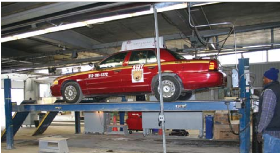
The 30,000-lb capacity four-post lift found at the City of Chicago’s Department of Consumer Affairs testing facility.
