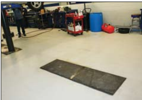
An extra lift built into the floor at Family Hyundai that can be fitted with locking bars and cylinders if needed.
