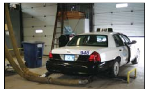
A cab uses a dynamometer in order to test its fare meter, ensuring that the customer is charged a fare price.
